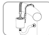
If you don't have a wall skimmer: 4 connectors (**G1/G2/G3/G4**) are provided in the kit to fit the 7 most common types of strainer (see below) used in above ground pools. According to the strainer used in your pool, select and attach the correct one to the strainer. Tighten by hand only.
