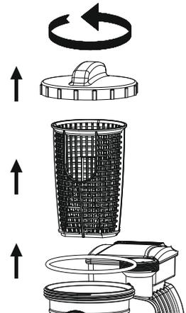
**NOTE:** The Strainer must be emptied and cleaned periodically. A dirty or blocked strainer will reduce the performance of the sand filter.
